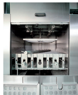
Service doors offer clear access to all components for easy maintenance.
